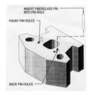
**Keystone's** patented pin system features high strength, pultruded fiberglass pins that provide a shear connector, geogrid proof positive holder, and alignment device all in one piece.
