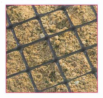
Ideal for reinforcing medium-small sized granular soils, having an aperture of 30x30 mm.
